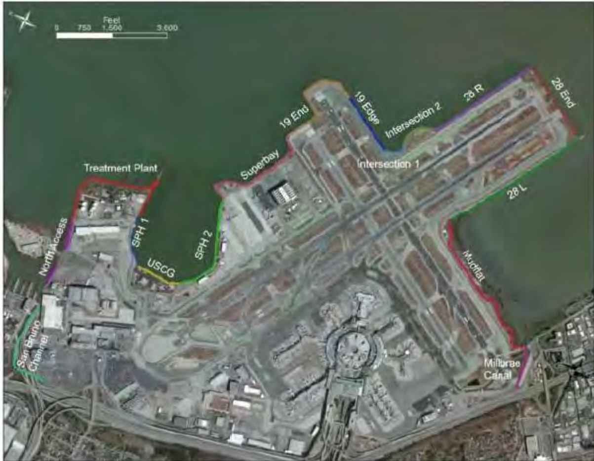
Figure 12: San Francisco Airport Shore Protection Structures
