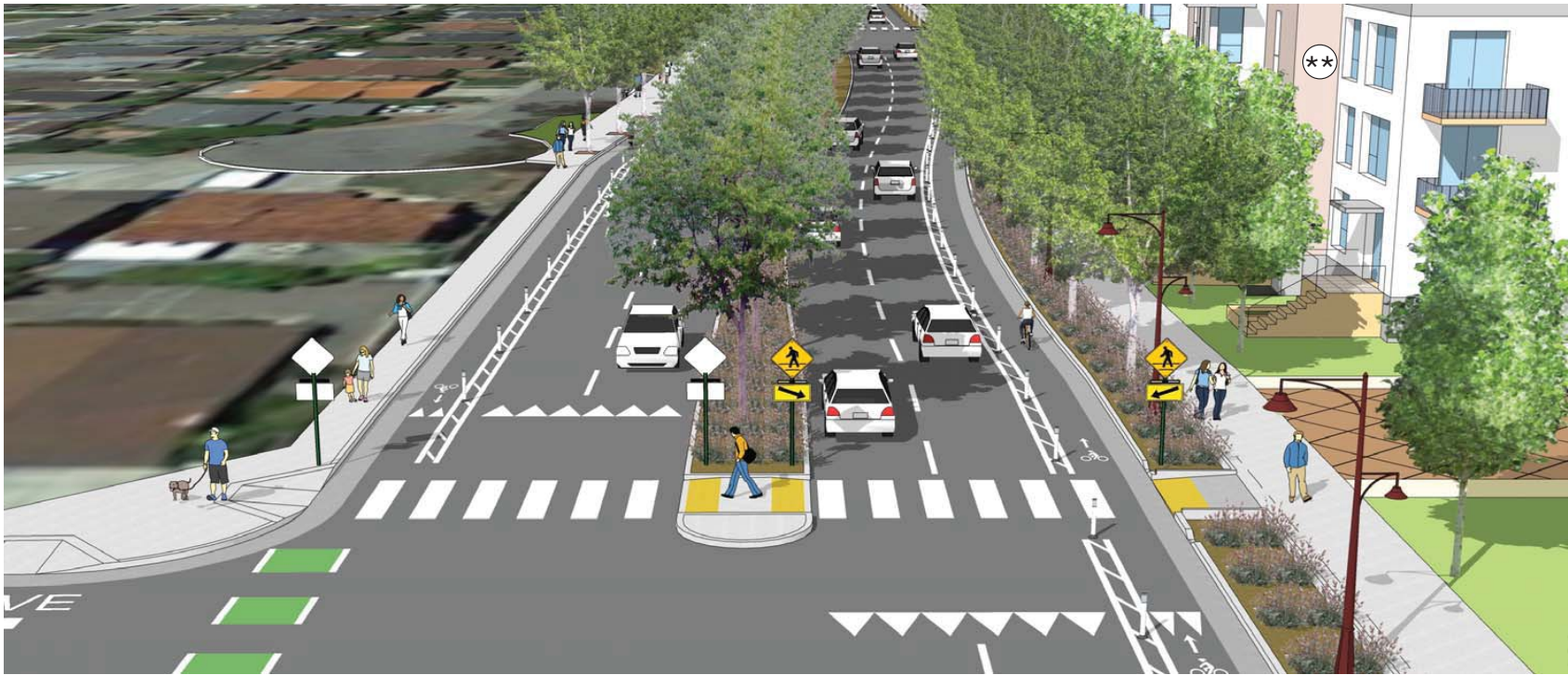
Figure A-24: San Bruno Avenue - Streetscape Concept with Buffered Bike Lane West
