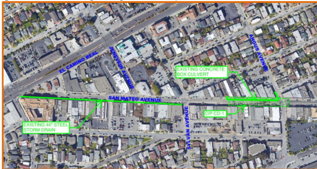
Figure 3: Storm Drain Capital Improvement Project Location
