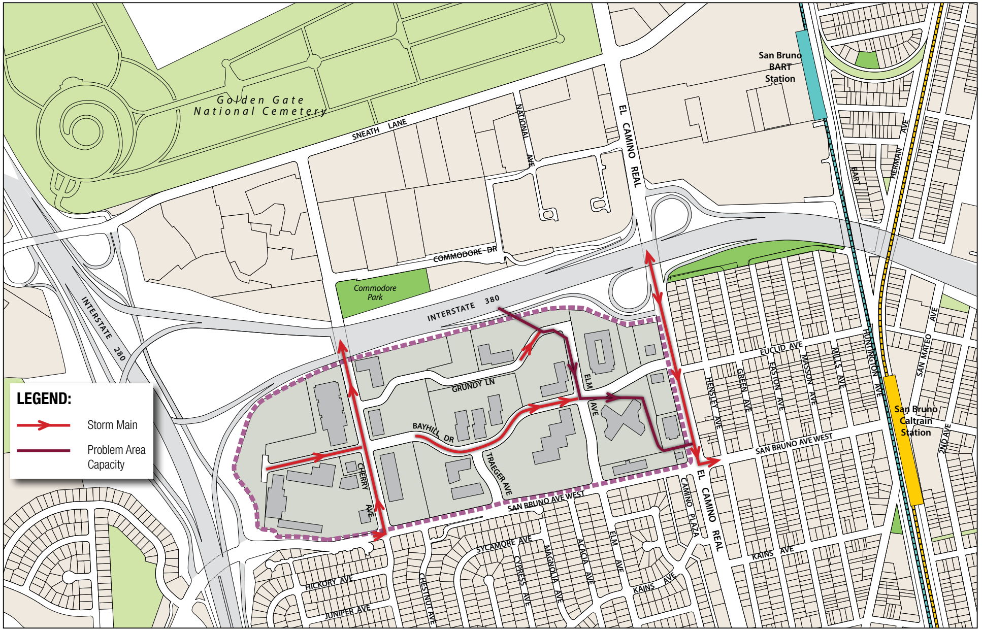
Figure 5-3: Existing Storm Drain System
