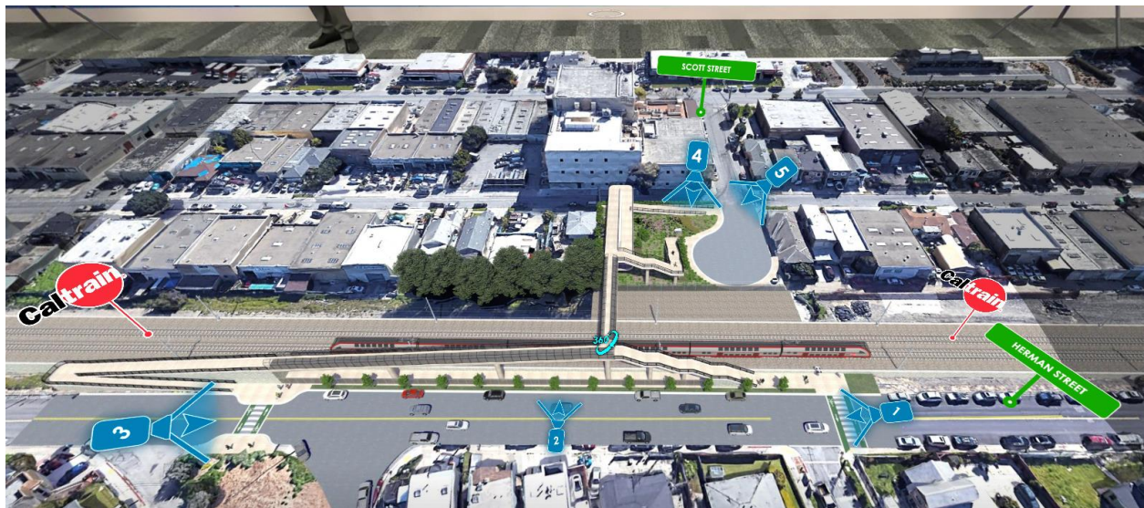
Three-Dimensional Model of the Pedestrian/Bicycle Overcrossing
