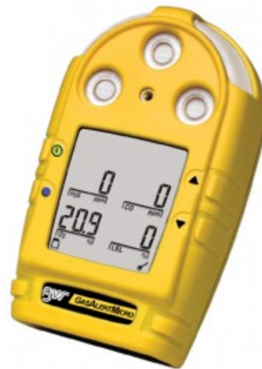
Photo 2. Typical Personal 4-Gas Monitor
